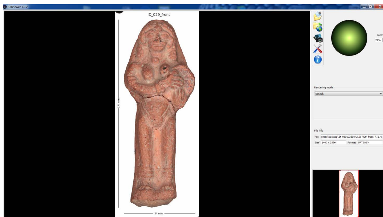
Fig. 3: The finished file loaded as displayed by the RTIViewer. The lighting angle can be manipulated using the virtual trackball (top, right), and a collection of visualization filters can be accessed via a drop-down menu (middle, right).
