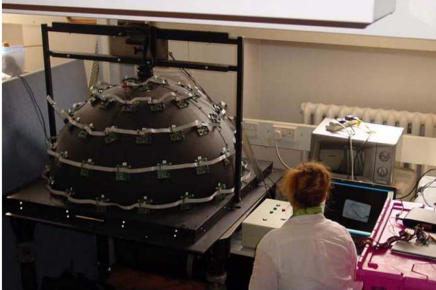
Fig. 5: An RTI-dome with 64 flash units
