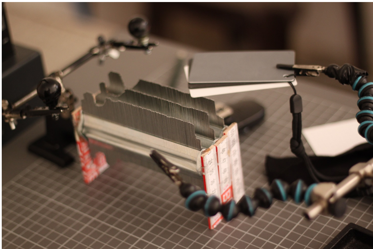
Fig. 7: A contraption made of aligned pottery gauges used as a fixture for the figurines.
